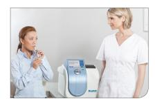
Your caregiver will connect you to a comfortable nasal breathing cannula. You will simply breathe normally for about 10-15 minutes, and the  $BreathID^{\otimes}Hp$  System will automatically sample your breath. In the middle of the test, you will be given a special, safe solution mixed in 5 to 6 ounces of water to drink through a straw.
